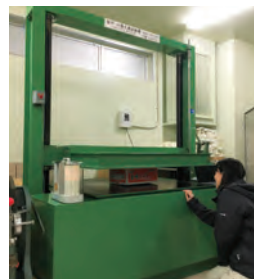
Quality checking of cardboard boxes using pressure testing equipment
