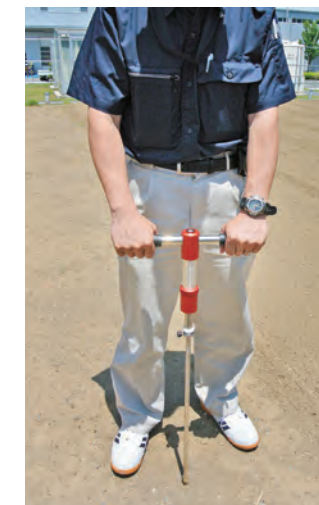
Measuring the hardness of soil using the ZEN-NOH physical properties diagnostics set
