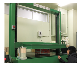
Quality checking of cardboard boxes using pressure testing equipment
