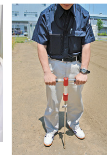
Soil physical properties diagnostics set
